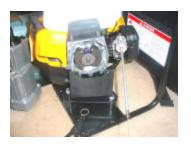
3) Using a snap ring pliers, remove the retaining ring, them remove the engine from the frame.
