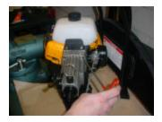
2) Remove the four socket head screws from the speed increaser.
