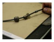
Feed the gray bushing over conduit. Feed the wires through the end cap; make sure the swivel slot is towards the end.
