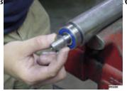
Clamp the rib of the rotor in a vise. Unscrew the driver sleeve (left hand thread). Remove the spacer from the rotor. Unscrew the hex nut from the opposite end of the rotor (left hand thread). Remove washer, the remaining two
