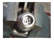
Looking into the motor housing you can see the internal lock ring on the motor seal. With a pair of lock ring pliers compress the lock ring and remove.
