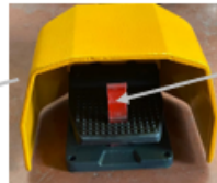
FOOT PEDAL – safety lever must be pushed fully back while pressing foot switch to operate.
