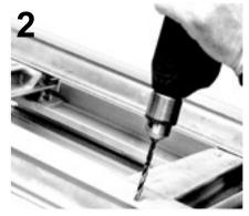
After repeating step 1 on opposite base rail, use bit in parts bag to drill all four holes. Use center punch if needed.
