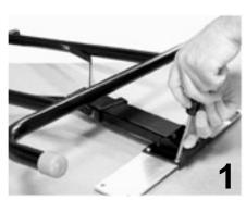
Using the sheet metal screws provided, attach mounting plates to leg strut flanges as shown. Turn brake over and rest each leg assembly onto base rails with the mounting plates extending toward center of brake.
