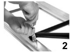
Locate holes in bottom of base rails toward each end of the brake and align with holes in U clamp. Position leg tube ends within clamps and tighten using slotted hex screws provided.
