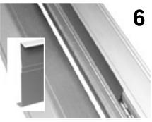
Complete fascia profile by removing piece from brake and reinserting with the finish side down and the top edge extending outward from the brake. Bend top leg until it matches roof pitch.
