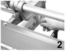
Tighten thumb screw to lock the stop block in place. Repeat tightening of opposite stop block and recheck measurements using the tape rule.
