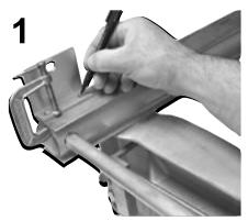
Turn brake over and line up wheel bracket with corner of base rail. Clamp in place and use pencil to mark holes.
