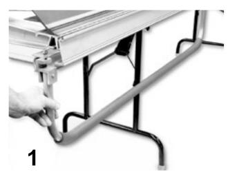
The bending handle assembly shown above comes with handle brackets which are pre-installed. Back off thumb screws far enough to clear front hinge flange and slide assembly onto front hinge. Tighten thumb screws firmly once handle is in desired position. To adjust handle position, loosen both thumb screws, move handle to new location and tighten thumb screws.
