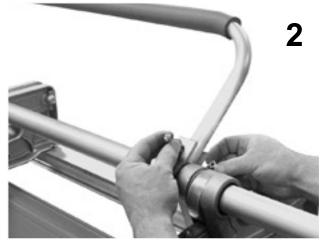
Place handle ends into bracket openings and align holes in brackets with holes in handle. Insert screws through holes and tighten snugly with hex nuts. Once you have both handles in place, the brake is ready for use.
