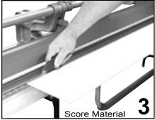
Lay out material from coil and score along desire trim length\*. Next, score along desired width. Transfer the bending information to the scored material ("blank"). With the finish side of the material as your reference, remember to indicate bends up and bends down
