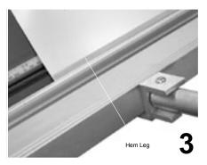
Remove material from brake and re-lock clamping surfaces. Place hem edge between vinyl strip and stainless edge. With one hand maintaining piece in position, Bend hem leg snug to material.
