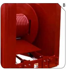
Shown with cable pressure bar and grooved drum modification.
