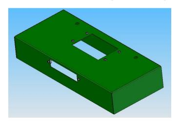
2. Install lower shroud of Power Flanger unit (A) using the four 1/4-20 x 1/2" long hex head screws. The back plate (C) should be inserted into the slots of the lower shroud.
