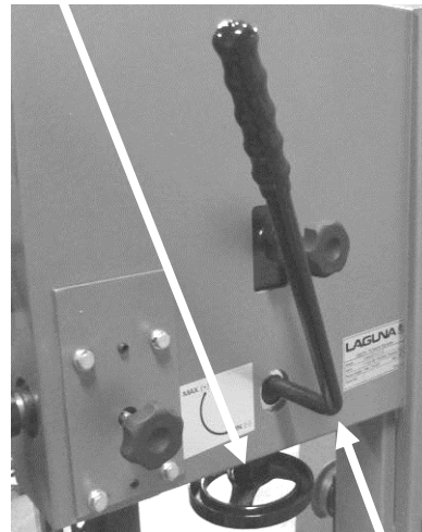
Quick action blade tension lever (activated)
