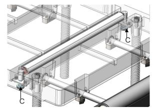
FIGURE 24: TABLE ROLLER ADJUSTMENT
