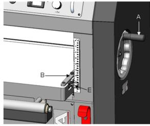
**NOTICE!** The following procedures describe the use of a "calibrating board". It is a piece of hardwood which has been surfaced on one side with a jointer, drum sander or wide belt sander.
