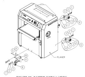
FIGURE 28: CASTER INSTALLATION
