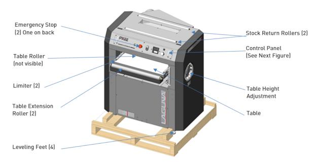
Figure 6: Main Components of PX22
