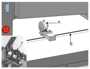
FIGURE 23: TABLE ROLLER ADJUSTMENT
