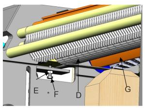
FIG. 18: INFEED ROLLER ADJUSTMENT
