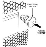
Figure 22. Start/Stop Switch (OFF Position)
