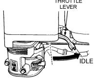
Figure 21. Throttle Lever (Idle)
