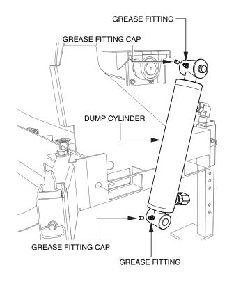
Figure 11. Grease Fittings (Dump Cylinder)
