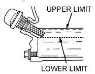
Figure 8. Engine Oil Dipstick (Oil Level)
