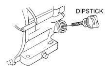
Figure 7. Engine Oil Dipstick (Removal)
