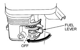
Figure 23. Fuel Valve Lever (OFF)
