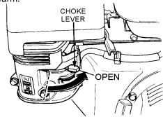
Figure 15. Engine Choke Lever (Open)
