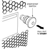
Figure 17. Start/Stop Switch (Start Position)
