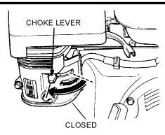
Figure 14. Engine Choke Lever (Closed)
