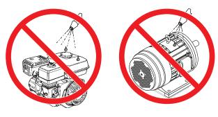
Figure 33. No Spraying of Water
