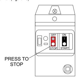
Figure 25. Electric Motor On/OFF Switch (Stop)
