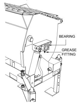
Figure 10. Grease Fittings (Bearings and Seals)
