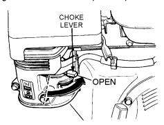
Figure 19. Choke Lever (Open)
