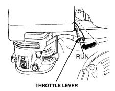
Figure 20. Throttle Lever (Run)
