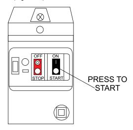
Figure 24. Electric Motor On/OFF Switch (Start)
