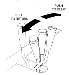
Figure 27. Hydraulic Dump Lever
