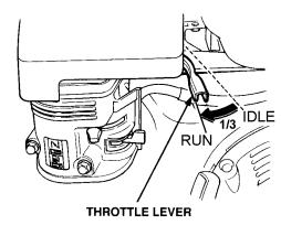
Figure 13. Throttle Lever (1/3 Start Position)
