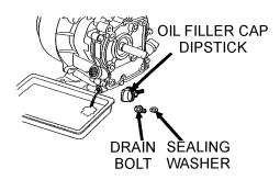
Figure 30. Engine Oil (Draining)
