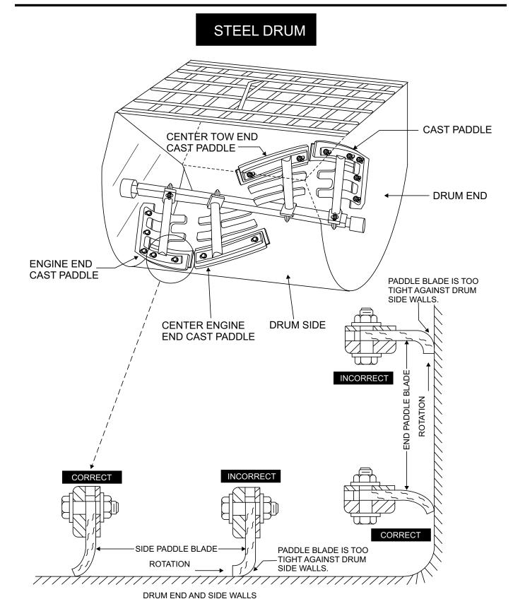
Figure 6. Paddle Blade Adjustment
