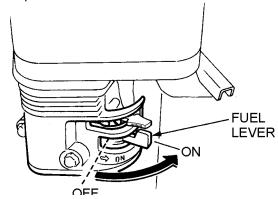
Figure 12. Engine Fuel Valve Lever (ON Position)
