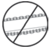
CHAIN TOO LOOSE
