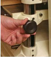
Cutting depth adjustments are made using the large cast iron handwheel (left) which also has a spinner handle built in to make large changes go quickly. A large knob at either end of the table (right) locks the height setting for precise, clean cuts.
