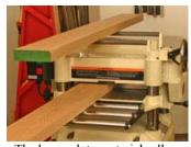
The heavy duty material rollers on top make returning heavy stock for the next cut easier and safer.
