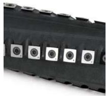
The carbide cutters on the helical head each have four individual edges. Should one edge go dull the inserts can be indexed four times, each producing a totally new edge.
