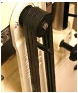
Motor power is delivered through a gang of three v-belts running in precisely machined pulleys.
