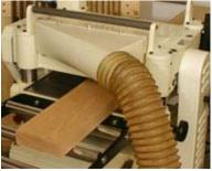
The 4"-diameter dust port is angle to the side to prevent the dust collector hose from interfering with the wood as it exits the planer.
