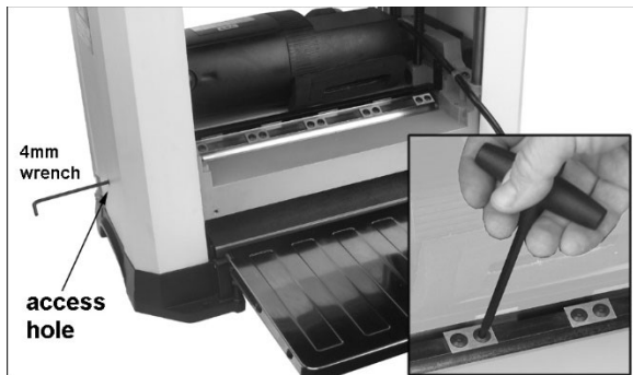
Figure 8-4: knife insert rotation/replacement
