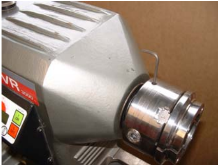
Removing grub screw to release insert
