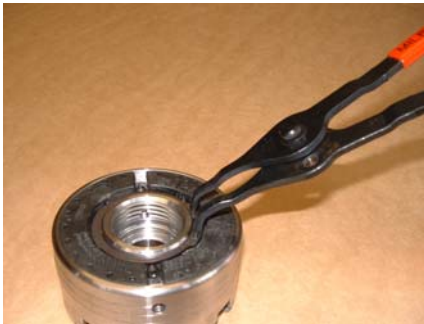
Using Circlip pliers to remove circlip
