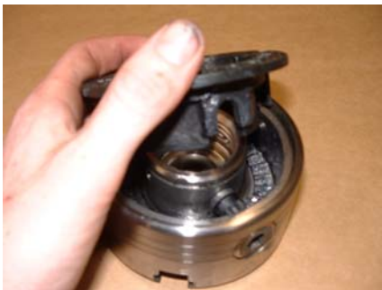
Lining up backing plate with pinions
