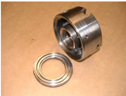
Removing scroll ring from Chuck
