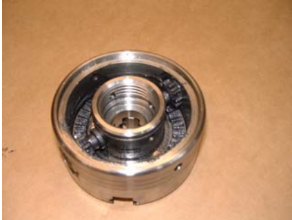
The Pinions can now come out by hand, as illustrated in the photo above.
