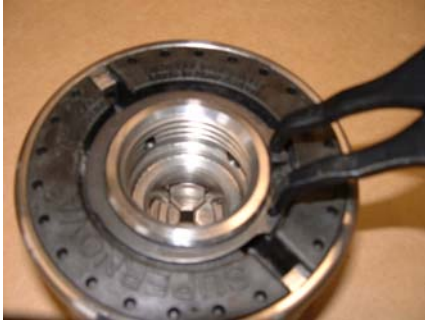
Showing circlip snapped closed
