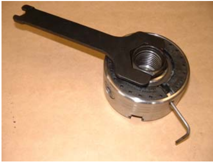
Using 1 1/2" spanner to re-attach insert.
