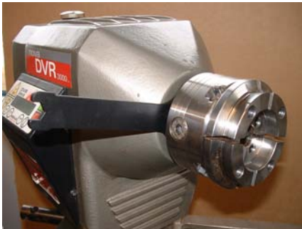
Using 1 1/2" Spanner to remover chuck from lathe
