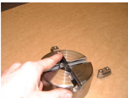
Removing jaw slides by hand
