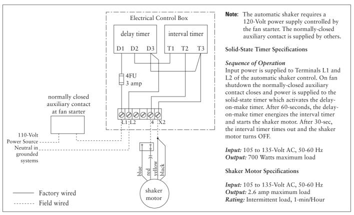
Seriec 50 to 80 Automatic Shaker without Transformer Wiring Diagram
