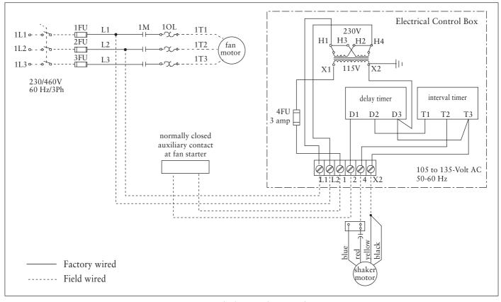
Seriec 50 to 80 Automatic Shaker with Transformer Wiring Diagram
