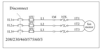
Motor Starter Wiring Diagram
