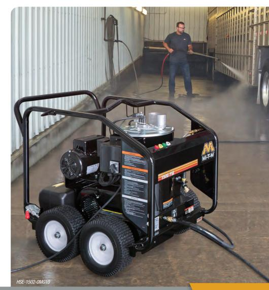
The HSE Series of direct drive hot water electric pressure washers are built for industrial cleaning on construction sites, farms, mining and oil fields. Known for their efficiency and longevity, they feature a top-fired heat exchanger that is completely accessible for troubleshooting.
