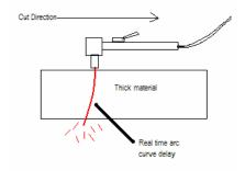
To avoid arc-curve delay, allow the arc to pass completely through the work piece before moving too far ahead. The arc-curve should lag not more than the thickness of the material being cut. In other words, if the work piece is one-half inch thick, the arc curve should lag not more than one-half inch behind the torch, as shown below.
